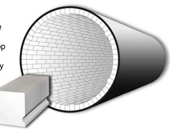
**Typical Composition of Alumina Brick:** Al<sub>2</sub>O<sub>3</sub> 90%, SiO<sub>2</sub> 6%, other 4%
