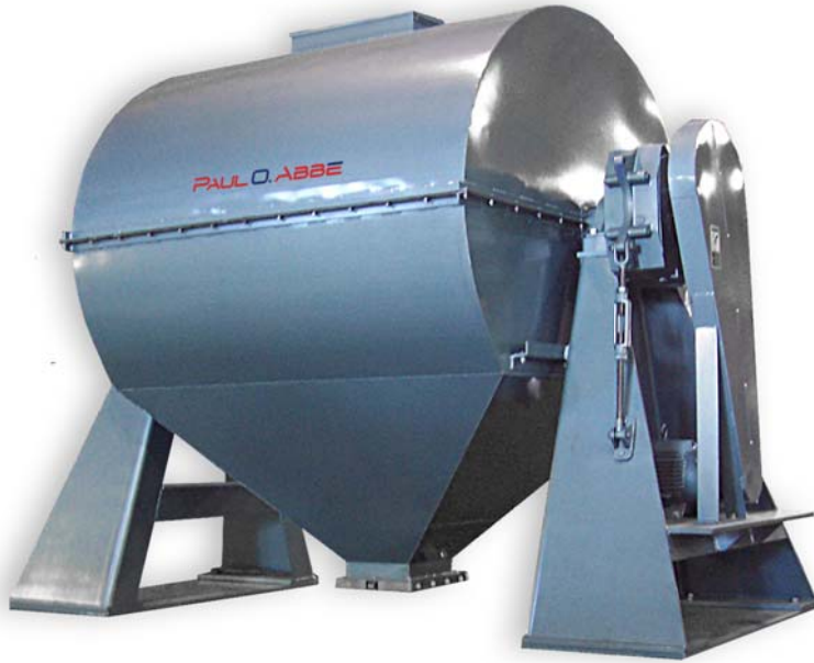
Shown above is a Full Housing which encloses the entire cylinder - dust seals are on the shaft.
