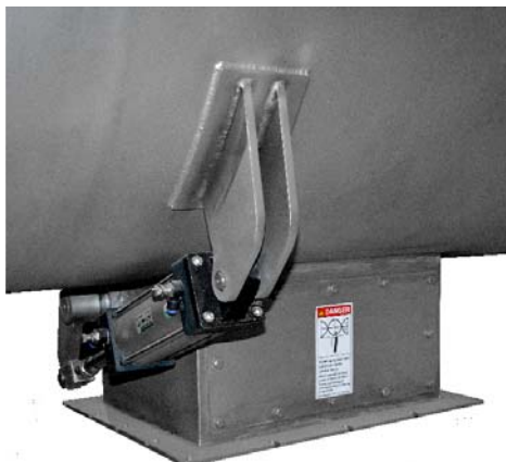
Discharge housing, pneumatic actuator, access panels (on both side of housing)
