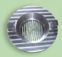
Dry Discharge Grate machined from stainless steel with 0.25" slots. The discharge grate retains the grinding media in the mill while allowing the finely milled solids to be discharged. In order to control the dust during discharge a dry discharge housing is recommended. Two designs of dry discharge housing are shown below.
