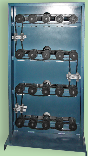
Synchronized Rollers: All 20 rollers on 4 tiers are driven at same speed from a single drive.
