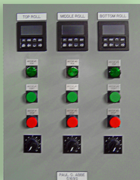
Independent direct coupled right-angle gear drives and separate speed controls and RPM readout for each tier.
